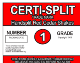
Figure R905.8.9 WOOD SHAKE DESCRIPTION AND EXAMPLE LABELS
