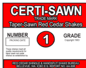
Figure R905.8.9 WOOD SHAKE DESCRIPTION AND EXAMPLE LABELS
