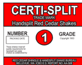
Figure R905.8.9 WOOD SHAKE DESCRIPTION AND EXAMPLE LABELS
